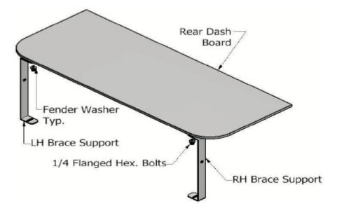
6. Mount the back support brace to the back of the drawer. Note: If the vehicle is a commercial vehicle a rectangular cutout is required for the base of the back support to mount to the floor of the trunk area. The size of the rectangle cutout should be 4" wide x 4" deep and centered at the very back of the removable trunk mat. (See diagram below. The drawer has been omitted for clarity).
