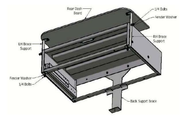
8. Place bolts thru the brace support brackets and tighten completely. Tighten brace support brackets that mount to the rear dash. (See Diagram above)
