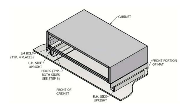
5. Locate the four holes on the back panel inside the cabinet assembly. Mount the cabinet assembly, through either hole to back metal framework vehicle, using at least one of the self-tapping screws supplied. (See diagram below. Uprights have been omitted for clarity.)
