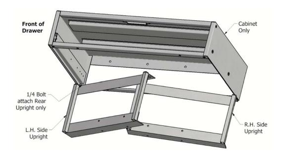
Slide the cabinet assembly all the way to the back of the trunk compartment and position the assembly between the wheel wells. Swing the uprights outward and attach them to both sides of the front of the cabinet using 1/4" bolts. (See Diagram below)
