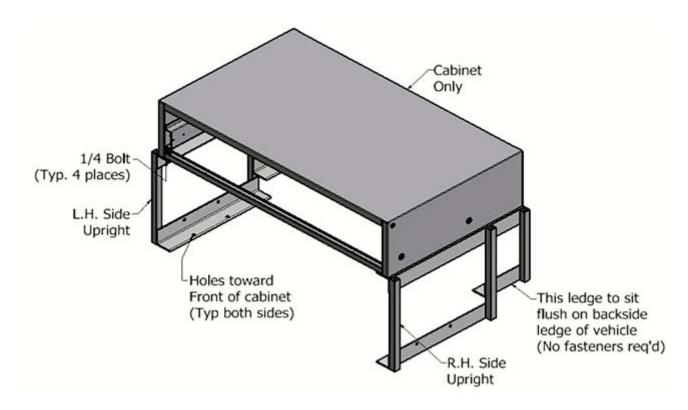
4. Locate the two holes on the bottom of the uprights and use the self-tapping screws to secure them to the trunk floor. Because of the gas tank location, wiring, hoses, etc, it is recommended that there be no additional drilling in the mounting zones. (See diagram below. The drawer has been omitted for clarity.)
