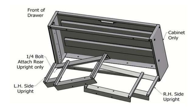
3. Slide the cabinet assembly all the way to the back of the trunk compartment and position the assembly between the wheel wells. Swing the uprights outward and attach them to both sides of the front of the cabinet using 1/4" bolts. (See Diagram below)
